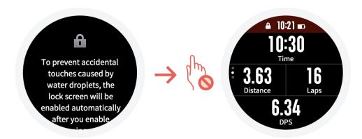
To protect the screen from unintentional touching and water interference, the watch will disable touch screen functions after you start swimming. During this time, you can use the watch buttons to operate. The watch will re-enable touch screen functions after you finish swimming.
