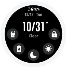
Swipe up on the watch face or short press the DOWN button to switch between Health status → Heart rate measurement. Keep swiping up to return to the shortcut control screen → watch face.
